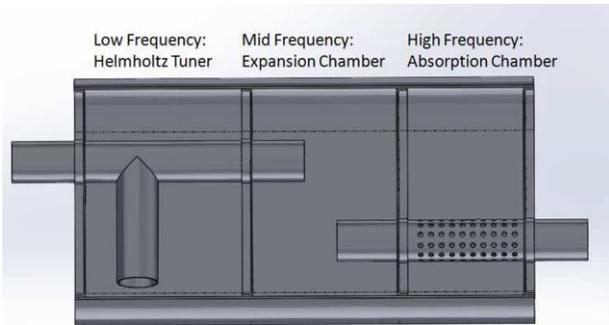
**Figure 3: 3-D manufacturing model created with modular parameters.**
