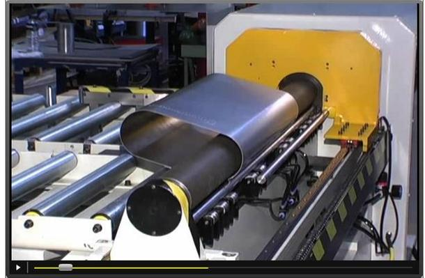
**Figure 4: CNC roll forming a muffler shell.**
